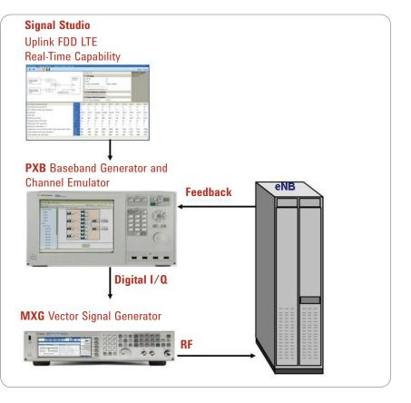
FIGURE 1: The PXB combined with the MXG and Signal Studio software enables efficient LTE eNB conformance testing.
